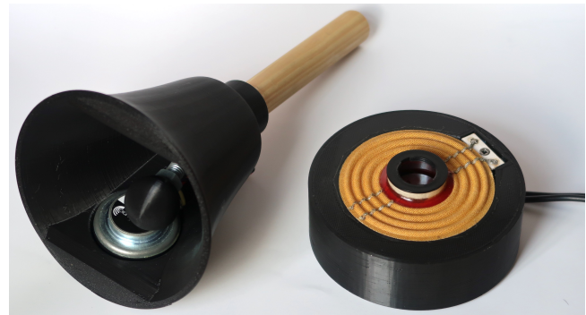
Figure 1: Haptic feedback instrument interfaces that each use a single voice coil transducer for both sensing and actuation.
